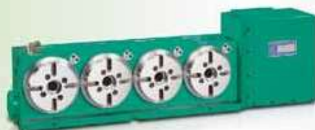
NCT-125-T2,T3,T4 CNC Multi-Spindle Rotary Table
