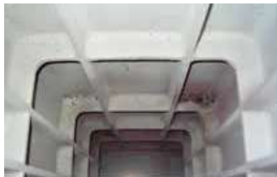
Fig. 1 Casting with heavy ribs (sample from model V26)
