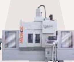
TT-40 Bridge type Twin-table VMC
