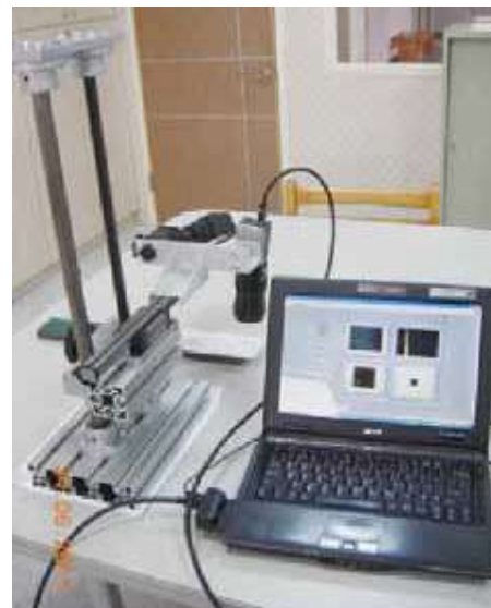
Fig. 9 Prototype of a scraping guide ways inspection device
