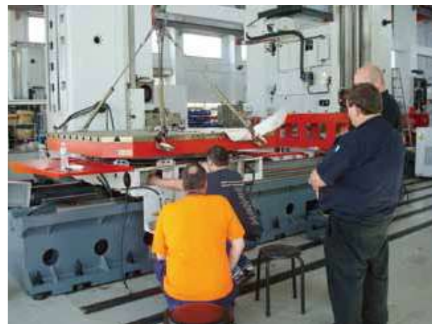
Photo story: Mr. Darren Goldring tried to assemble the worm shaft of table transmission system. Table was just re-assembled on this machine.
