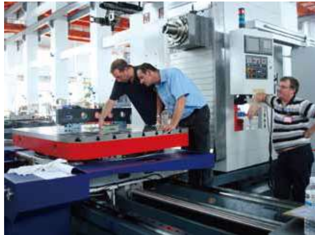
Photo story: Mr. George Buchel from company VOLZ and Mr. Anton Rusche from company Franz Moser are kneeling on table to check table leveling.
